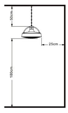
2. Now attach the supplied fastening chain to the holder hook by hooking one end of the chain into the holder hook with a carabiner.
